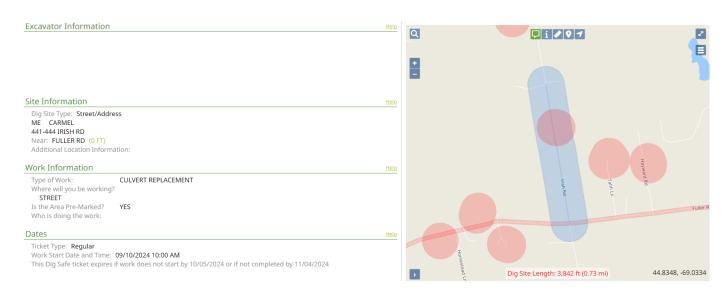
If the **BLUE** highlighted area (proposed area of excavation) overlaps with the **PINK** highlighted area (member facilities underground data), the member company will get notified (i.e. receive the Dig Safe ticket).
